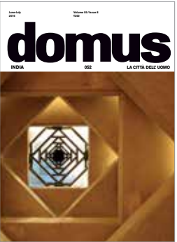
Cover: Rather than a solid block, the individual components of the shikhara of the temple in Barmer, Rajasthan designed by SpaceMatters, are offset from each other. This helps channelise more light into the inner sanctum or the garbhagriha of the temple. Seen here is the detail of the vedika or finial, when viewed from below.
